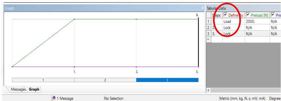
Figure 5. Adjustment of the time course of the screw preload
