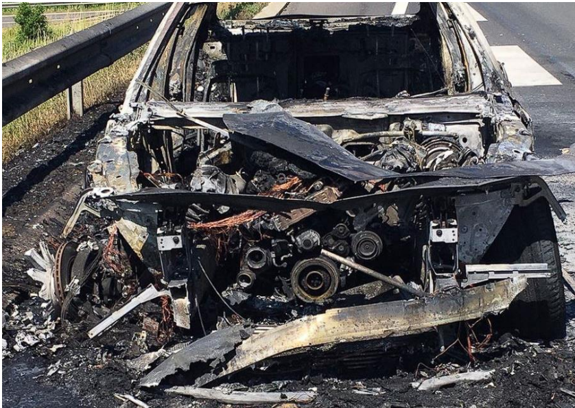
Figure 2. Vehicle with N47 engine after catching fire
