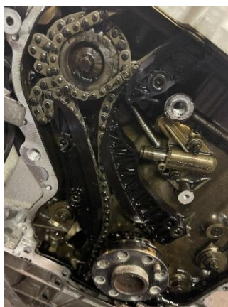
Figure 1. Timing chain failure (break)
