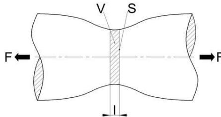
*Figure 1. Characteristics of the un-notched and notched specimens* [10]
