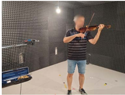
Figure 5. The measurement setup in semi-anechoic chamber
