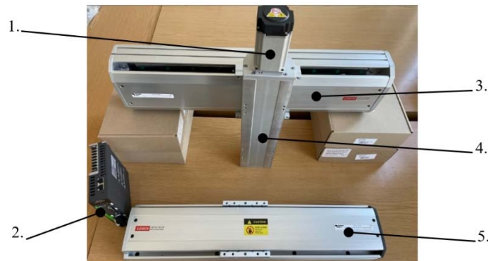
Figure 1. The linear units (3. – 5.) and one of the motors, motor drivers (1., 2.)
