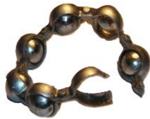
Figure 6. Failure of cage
