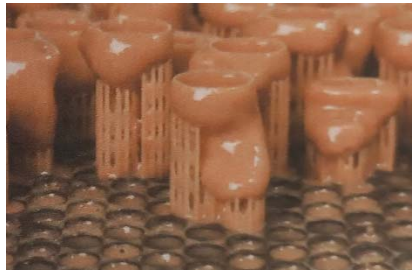
Figure 3. 3D printing with a large amount of support (hearing implant) (Gibson, Rosen, Stucker, & Khorasani, 2021)
