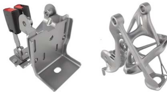
Figure 4. Car seat-belt bracket (traditional and generative design, 40% lighter and 20% stiffer) https://www.autodesk.com
