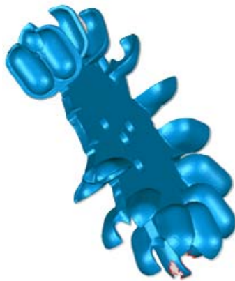
Figure 5. Scanned 3D geometry of impeller
