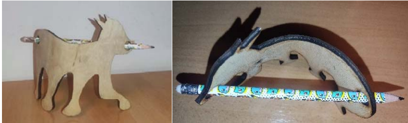
Figure 14. Fox hair ornament produced by steam bending
