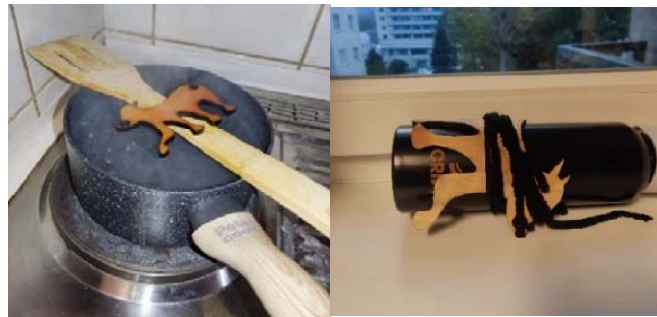
Figure 12. Steam bending process
