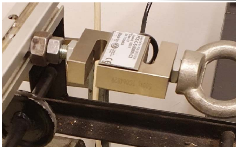
Figure 10. Force gauge in installed condition
