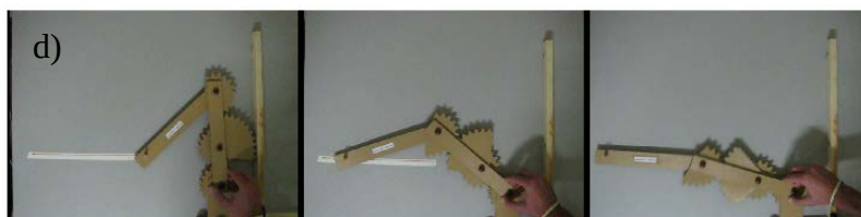
Figure 17. Open kinematic chain with linear motion of the free end
