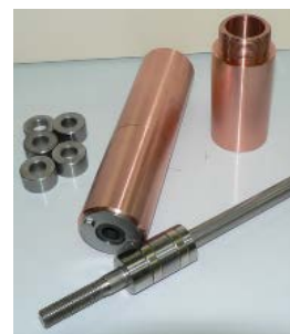
Figure 3. Principle of the EM damper – drawing and testing prototype photography
