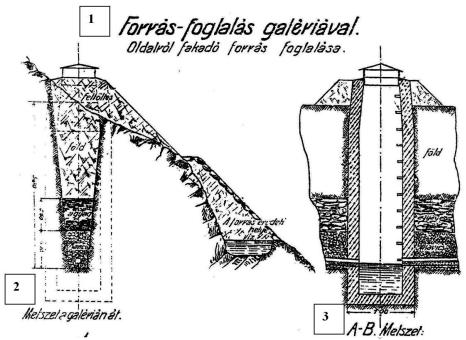
Figure 4. Fragment from original project documentation depicting capturing of Čermel' springs. (1 - Capturing by a gallery; 2 - Cross-section of a gallery; 3 - Section A-B)
