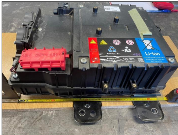
Figure 1 Unassembled Ford Transit battery pack
