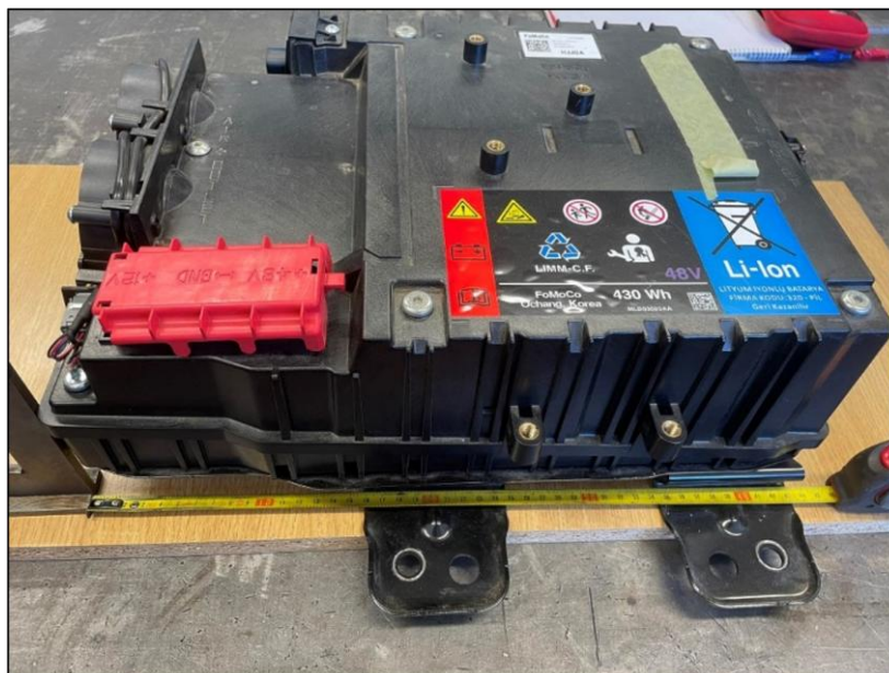
Figure 1 Unassembled Ford Transit battery pack
