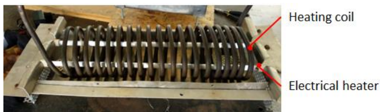
Figure 3 The heating coil of the steam generator
