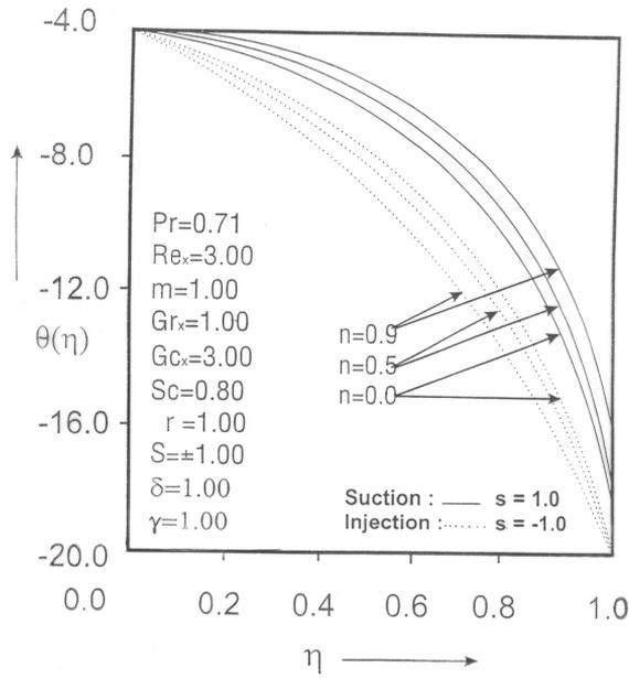
Figure 2. Influence of thermal stratification over the temperature profiles
