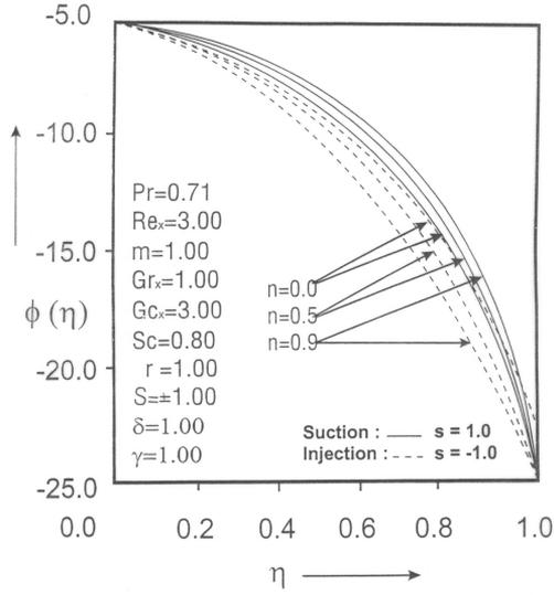
Figure 3. Effect of thermal stratification over the concentration profiles
