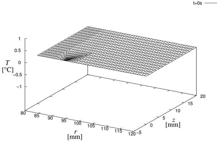
Figure 10. The approximated temperature distribution of the upper body at  $t = 0$  s
