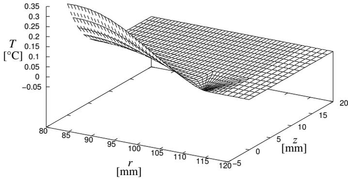
Figure 14. The approximated temperature distribution of the upper body at  $t = 1$  s
