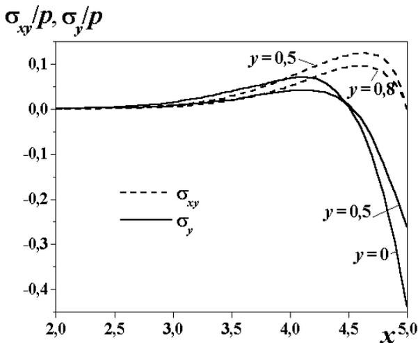
Figure 3. Behavior of the stresses  $\sigma_y/p$  and  $\sigma_{xy}/p$  for  $a = 5$  and  $b = 1$  a constant compressive stress along the region's width, which is equal to  $\sigma_x^0/p = -2/3$  according to the elementary solution.
