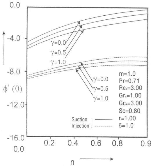
Figure 6. Influence of chemical reaction over the rate of mass transfer profiles
