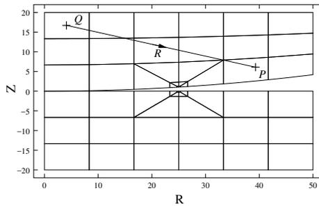
Figure 2. Let  $R$  be a ray that starts from the point  $Q$ , and passes through the elements to the point  $P$ .  $R$  crosses a side of the element containing  $Q$ , and enters the neighboring element. This neighboring element is the first in the further search process.
