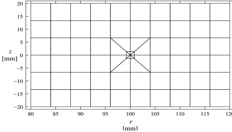
Figure 7. The finite element mesh of the cross-section of the bodies. The contact surface is the  $z = 0$  plane. The boundaries of the contact region are the  $r = 80$  mm edge and the point where the smallest element is situated, i.e.,  $r = 100$  mm
