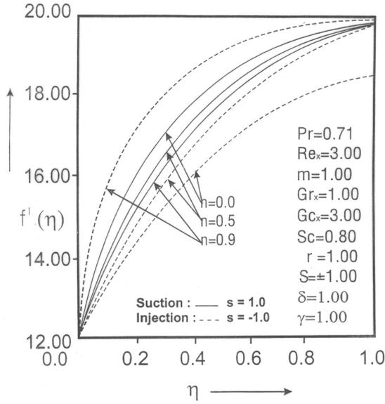
Figure 1. Effect of thermal stratification over the velocity profiles
