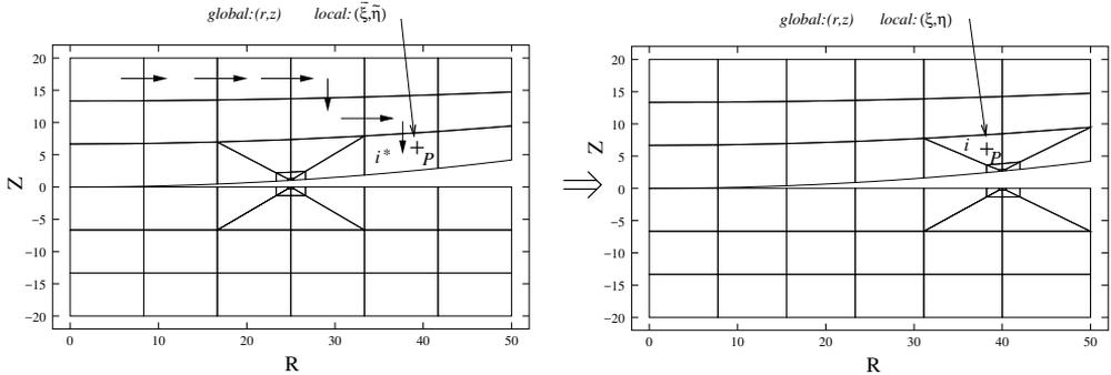
Figure 1. If element  $i$  and point  $(r, z)$  are known, the appropriate element  $i^*$  and local coordinate  $(\tilde{\xi}, \tilde{\eta})$  are sought on the old mesh.
