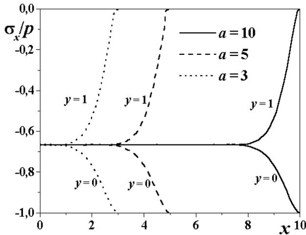
Figure 1.  $x$ -distribution of the stress  $\sigma_x/p$  for  $a = 10; 5; 3$  and  $b = 1$
