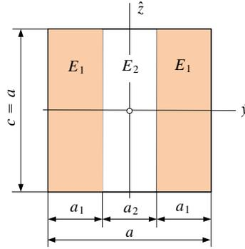
Figure 14. The cross section of an FrsRp beam
