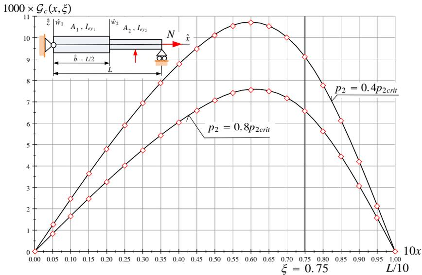
Figure 7. The Green function of a PPStp beam subjected to a tensile force
