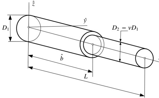
Figure 4. Stepped beam with circular cross section
