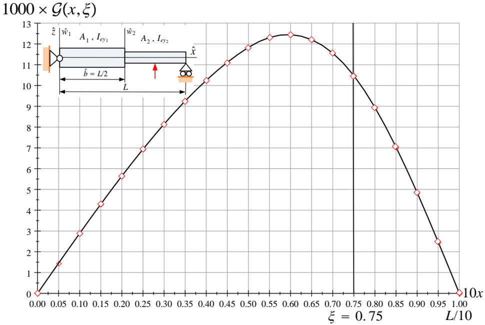
Figure 3. The Green function of a PPStp beam
