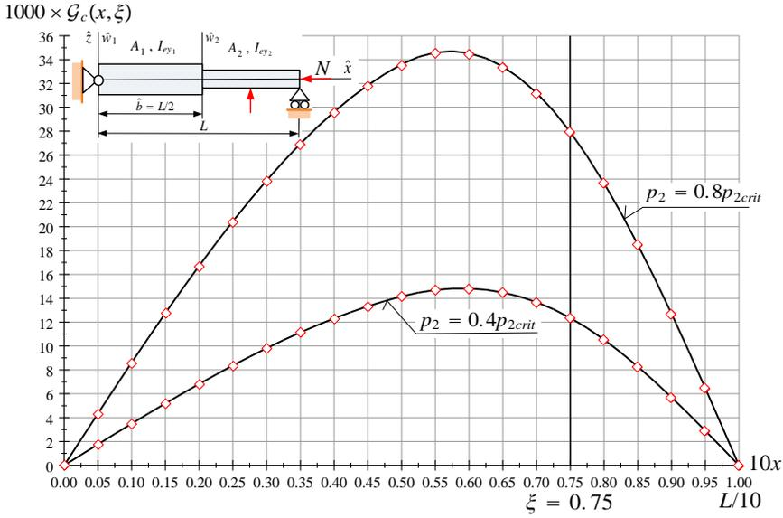
Figure 6. The Green function of a PPStp beam subjected to a compressive force
