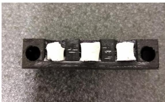
Figure 3. The samples in the mould after drying
