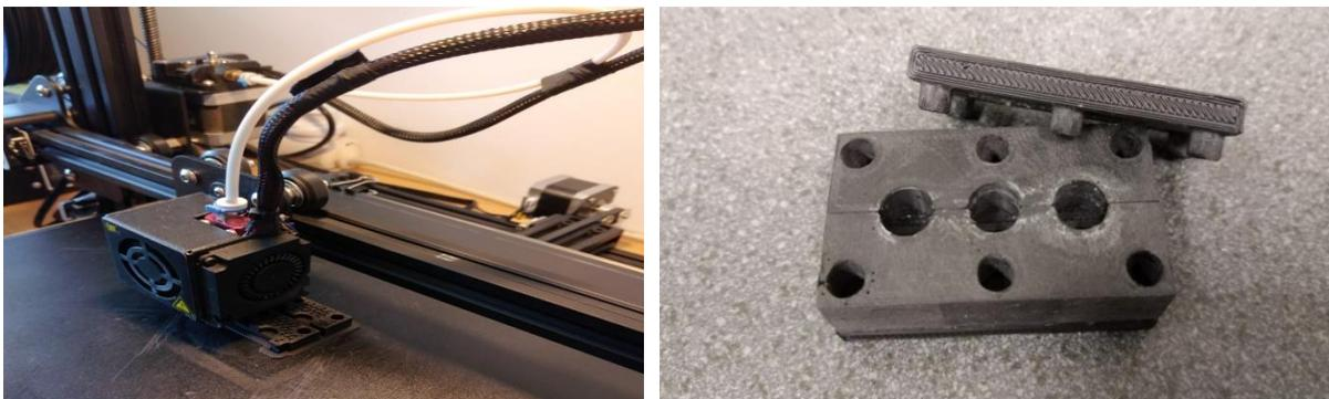
**Figure 2.** The 3D printed test mould
