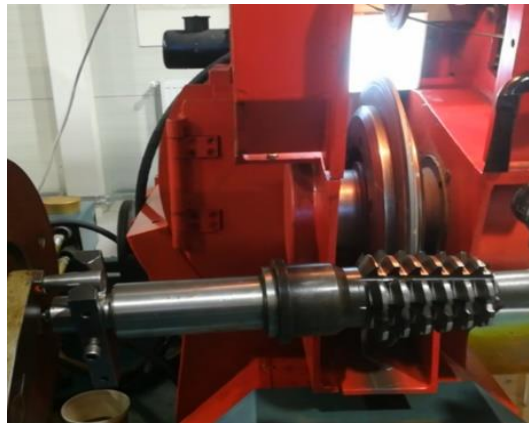
Figure 2. Driving with a counter-conical motion transmitter pin in the case of the conical hob machining in the DifiCAD Ltd. Engineering Office.
