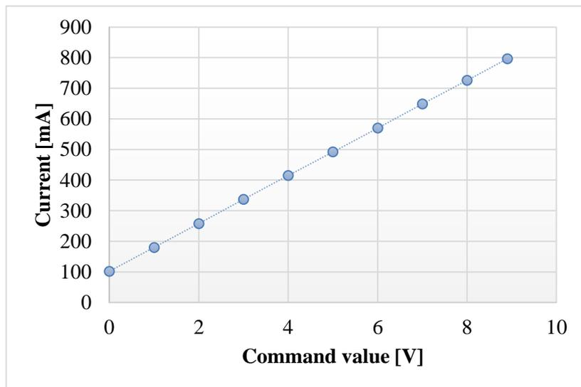
*Figure 5. Command value vs current of the valve's solenoid*
