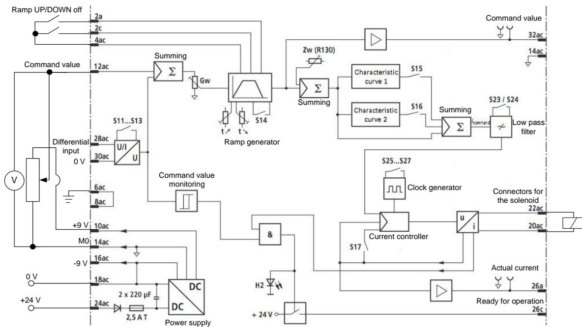
**Figure 2.** The elements of the proportional amplifier module and its wiring for the measurement
