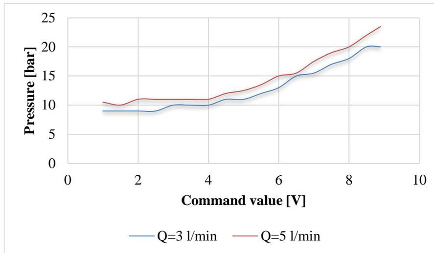
**Figure 6.** *Command value vs pressure at constant flow rates*
