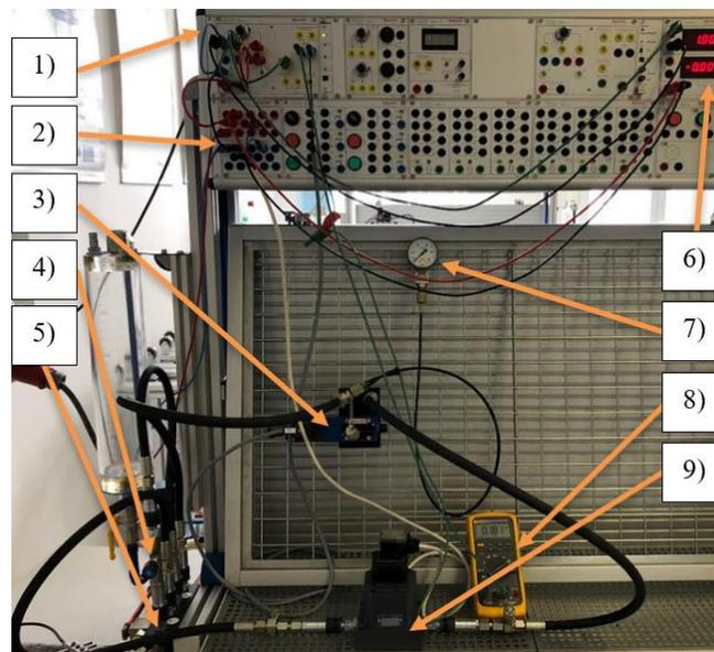
**Figure 4.** *Proportional valve unit under laboratory test*
