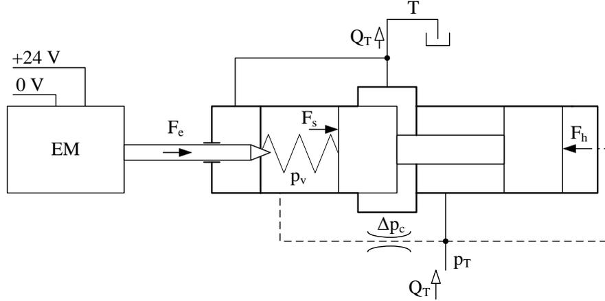
**Figure 1.** Schematic of the pressure relief valve
