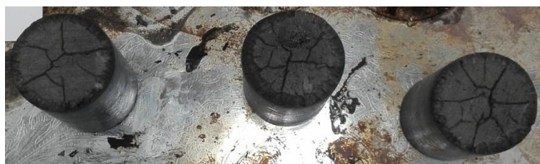
Figure 3. Cracks in GFA geopolymer composite specimens
