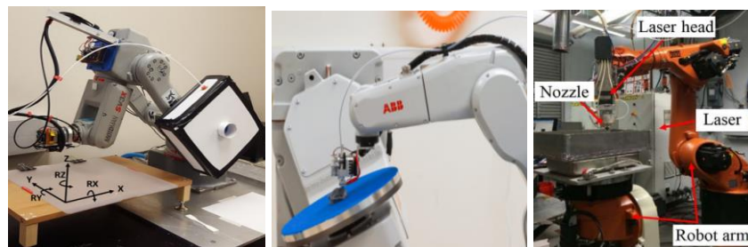
Figure 9. (left) representative set-up of multi-directional FDM platform (Ishak and Larochelle, 2019), (middle): 8-DOFs robot-assisted 3D printing system consisting of a 6-DOF ABB IRB1200-7/0.7 robotic arm and a 2-DOF IRBP A-250 tilting table (Dai et al., 2020), (right) Setup of the LBDMD system (Laser-based direct metal deposition) (Ding, Dwivedi and Kovacevic, 2017)
