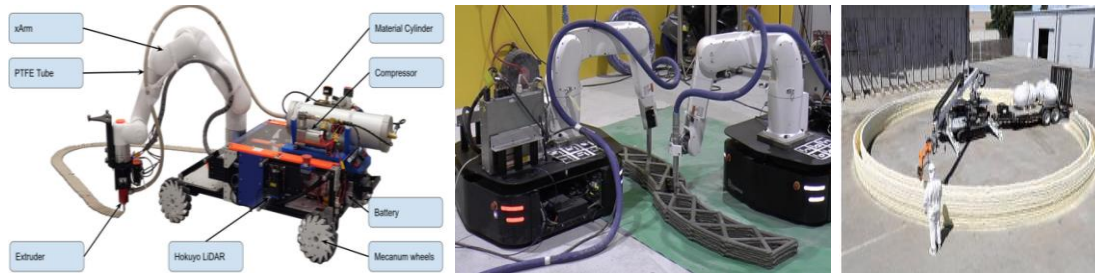
Figure 6. (left) Armstone robot's major components (two Intel Nuc computers and the xArm DC control box) (Sustarevas, Kanoulas and Julier, 2022), (middle) a large, single-piece, concrete structure by two mobile robot printers (Zhang et al., 2018), (right) Digital Construction Platform by a robot with a wide-range reach (Keating et al., 2017)
