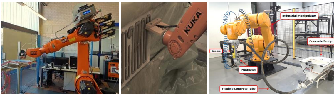
Figure 2. (left) present day view of Commissioned ARMS (Schwicker and Nikolov, 2022), (middle) 3DP of inorganic foams revealed onto walls (Lublasser et al., 2018), (right) a robotic arm construction 3D (Barjuei et al., 2024).
