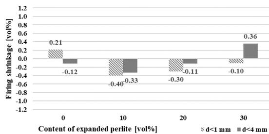
**Figure 8.** Firing shrinkage of samples containing 23 vol% sawdust
