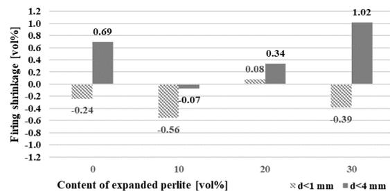
**Figure 9.** Firing shrinkage of samples containing 33 vol% sawdust
