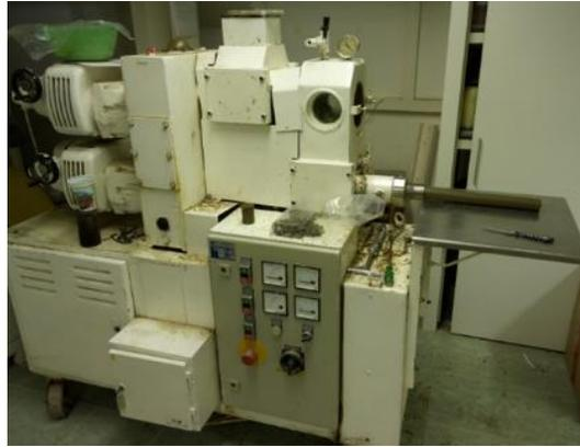
**Figure 3.** KEMA PVP 5/s laboratory vacuum extruder
