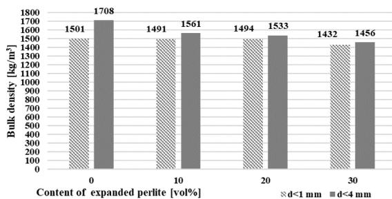
**Figure 10.** Bulk density of samples containing 23 vol% sawdust
