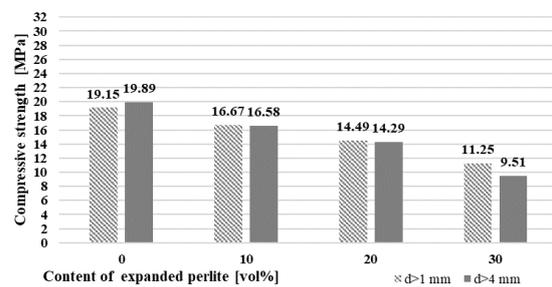
**Figure 15.** Compressive strength of samples (33 vol% sawdust)
