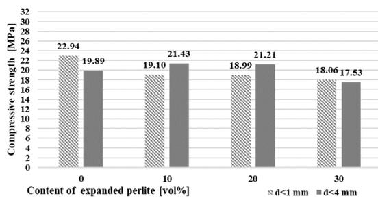
**Figure 14.** Compressive strength of samples (23 vol% sawdust)
