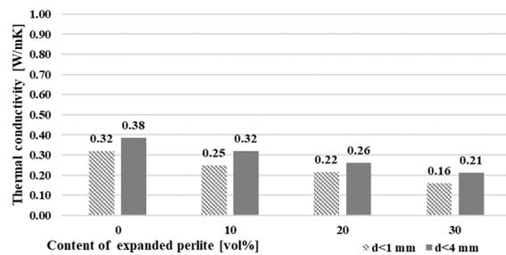
**Figure 17.** Thermal conductivity of samples containing 33 vol% sawdust
