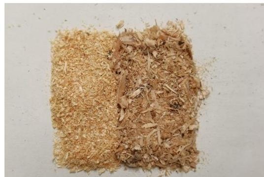
**Figure 2.** The sawdust fraction used as pore forming additive (left:  $d < 1$  mm; right:  $d < 4$  mm)
