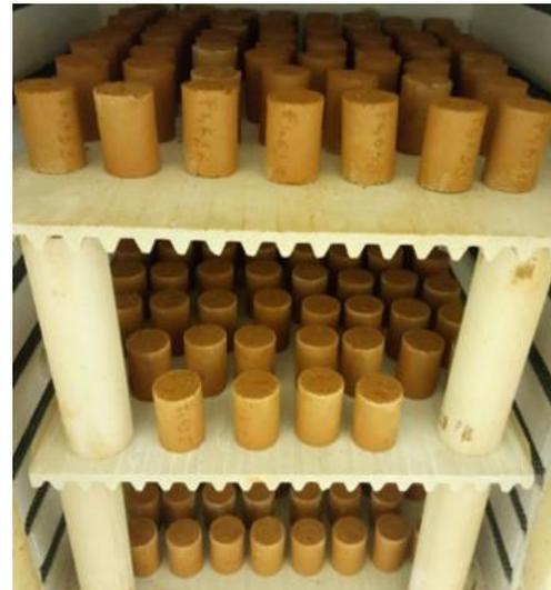
**Figure 5.** Samples fired at 870°C
