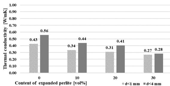
**Figure 16.** Thermal conductivity of samples containing 23 vol% sawdust
