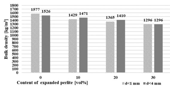
**Figure 11.** Bulk density of samples containing 33 vol% sawdust
