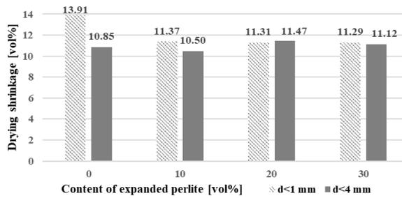
**Figure 6.** Drying shrinkage of samples containing 23 vol% sawdust
