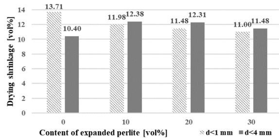
**Figure 7.** Drying shrinkage of samples containing 33 vol% sawdust
