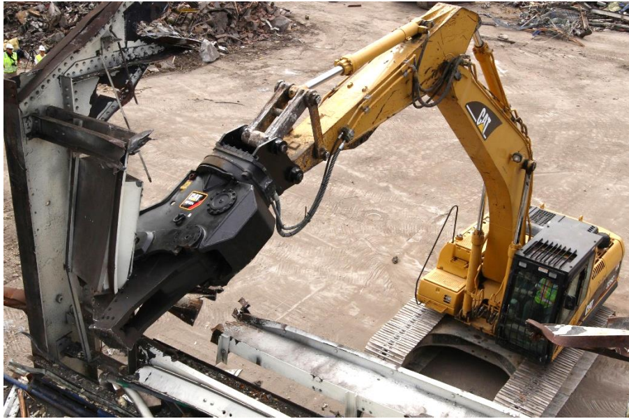
Figure 1. A typical hardfaced product is a demolition shear
