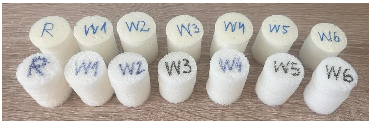
Figure 1. Flexible polyurethane foam samples for the mechanical and acoustic tests
