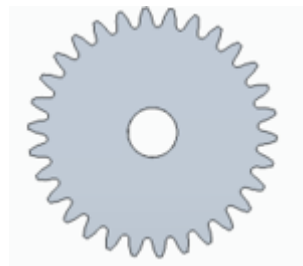
Figure 2. The 3D model of the m = 0.5 , z = 30 gear
