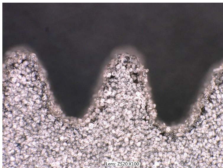
Figure 6. The tooth shape for m = 0.5 , z = 50
