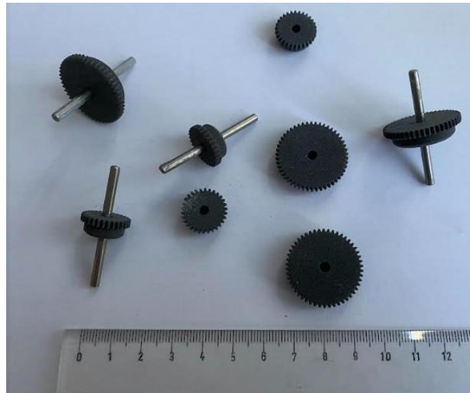
Figure 4. The 3D printed gears
