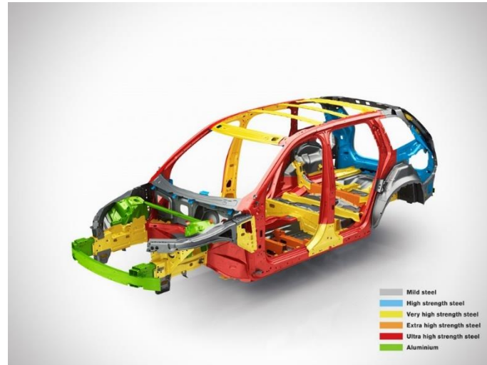
Figure 1. Body in white (BIW) colored schematic of Volvo XC90 (2019) (volvocars.com)
