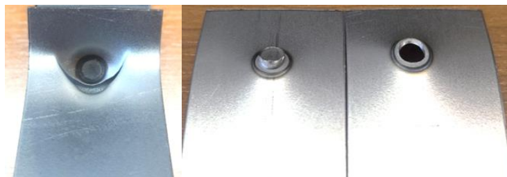
Figure 20. The failure mode in sample T1(plug-in base metal) is on the left and the failure mode in sample T3 (Plug) is on the right in DP600 samples
