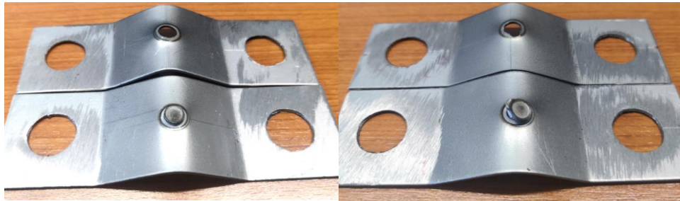
Figure 19. Plug failure mode in sample C1 is on the left and Plug failure mode in sample C12 is on the right in DP600 samples
