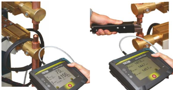
Figure 10 TECNA TE1700 RSW is current measuring using a flexible transducer prob on the left and a force measuring transducer prob on the right
