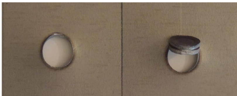
Figure 23. Plug failure mode in sample T10 of MS1400 samples
