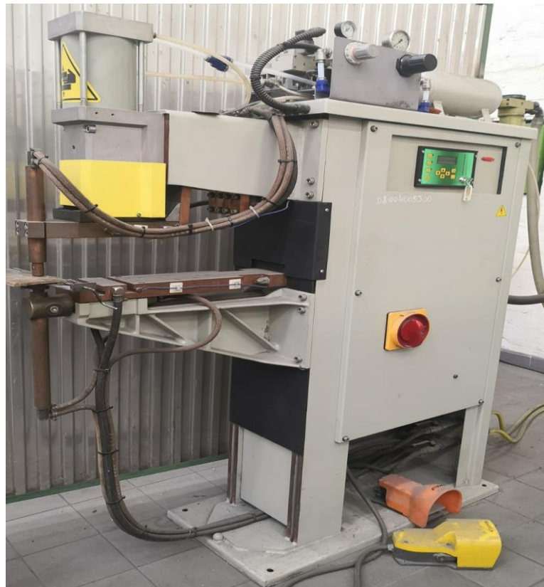
Figure 1. TECNA 8007 type resistance spot welding equipment
