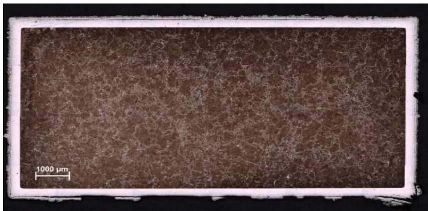
Figure 4. Mosaic optical microscope image of an aluminized C45 steel specimen
