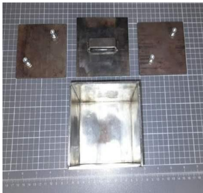
Figure 1. All parts of the reaction container
