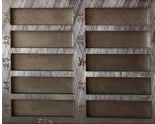
**Figure 2.** Test piece machined with EDM
