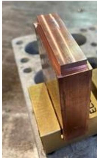
**Figure 3.** Copper electrode used for cutting experiments
