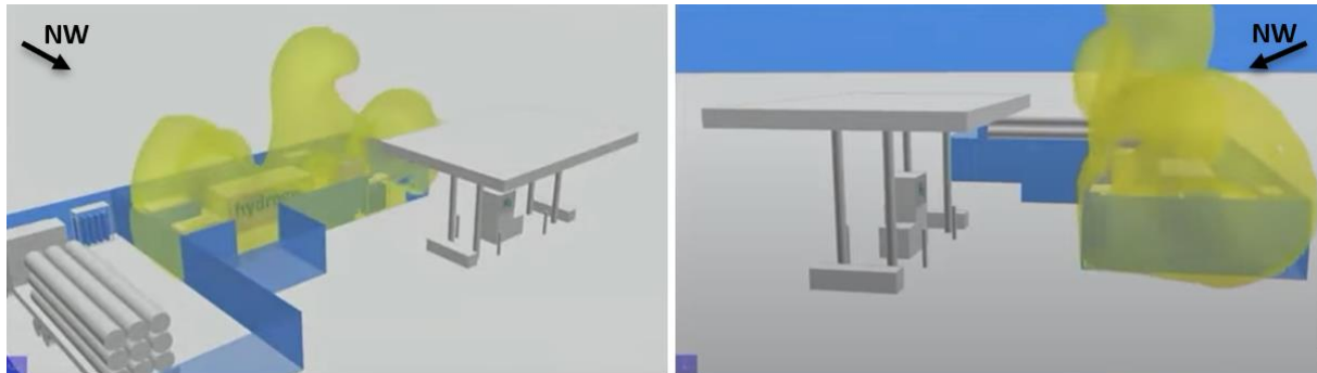
Figure 5. Hydrogen gas cloud propagation at 1 m/s wind speed (north-westerly direction)
