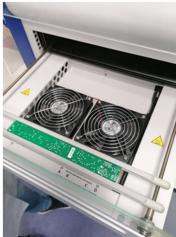
Figure 5. The PCB in the reflow oven
