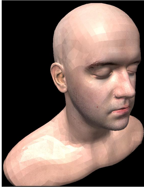
Figure 9. Head rendering with face level normal/tangent/bitangent attributes. The result is similar to flat shading
